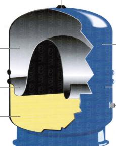
Durable steel tank Deep-draw steel shell for extra strength. A special welding process eliminates interior rough spots and sharp edges and prevents damage to diaphragm
